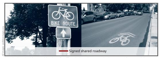
Standard road with a combination of traffic calming, signage and "sharrows" (shown at right), or a high-volume road with 14-foot or wider outside lanes.
